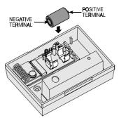
Use only Lithium Thionyl Chloride battery (Tadiran TL-5902 or equivalent).
